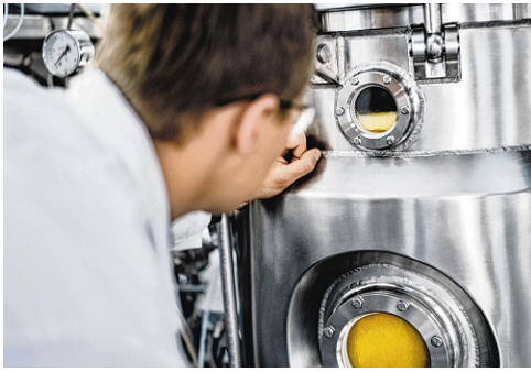
Solein being fermented in a bioreactor (right). The yellow microbe-based protein created by Finnish start-up Solar Foods can be used as the protein source for alternative dairy and meat, and also to raise the protein content of snacks, drinks, bread and spreads. PHOTOS: SOLAR FOODS
